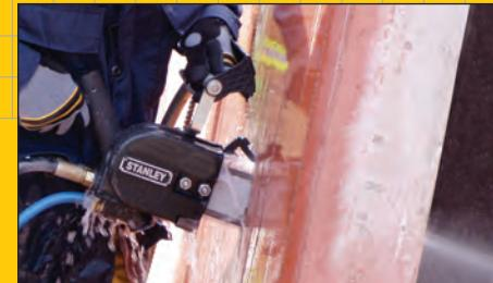
**DS06 Diamond chain saw - Bar length cm 33**Mod. DS06 3000 - flow 26-34 L/min - 140 Bar - EHTMA group **D** - Mod. DS06 300001 - CE Type - flow 26-34 L/min - 140 Bar - EHTMA group **D**Mod. DS06 200001 - CE Type - flow 15-23 L/min - 140 Bar - EHTMA group **C**
