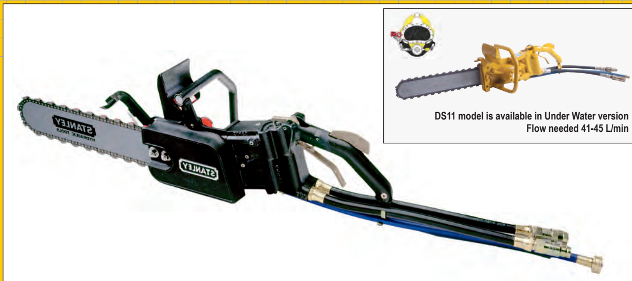
DS11 Diamond chain saw - Bar length cm 45 Mod. DS11 3000 - Flow 26-34 L/min - 140 Bar - EHTMA group D
